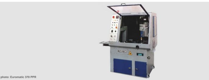
Fully automatic sawing machine working by hydropneumatic system.
